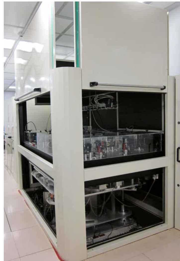
EIB in acoustic enclosure
