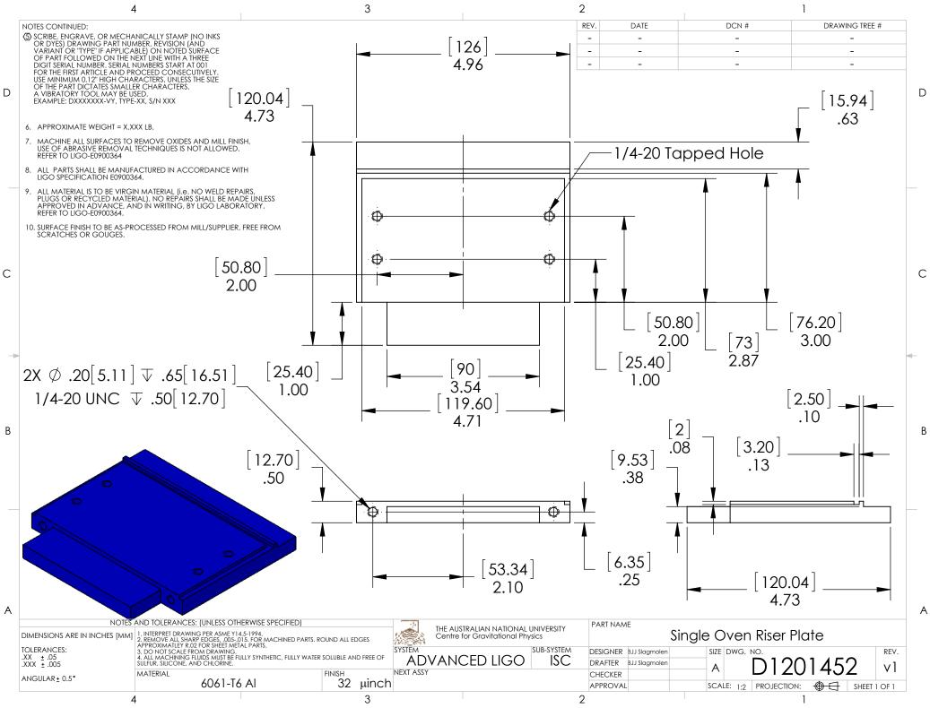
D1201452 Single Oven Riser Plate, PART PDM REV: , DRAWING PDM REV:
