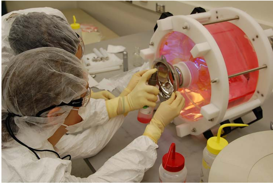
Figure 18. Person 1 holding cone while Person 2 sprays on an alignment layer
