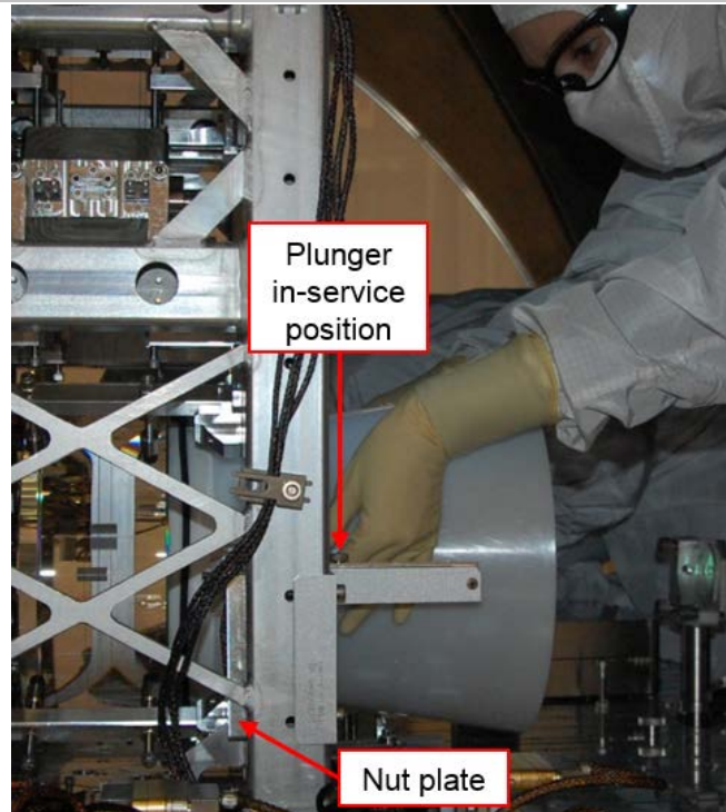
Figure 4. Adjusting thumb screws to move the cone to the in-service position on PR3 (side view)
