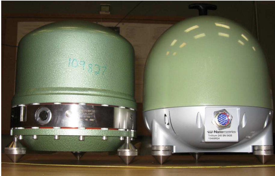
Figure B.1: The Trillium T-240 seismometer (right) next to the Streckheisen STS-2 seismometer (left). The T-240 is slightly taller but occupies a smaller diameter (as viewed from above). While the instrument diameters are similar, the T-240's feet are contained within the outer diameter of the instrument.
