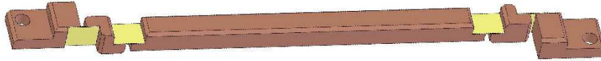
Figure A.8: CAD of the brass and BeCu flex strip flexure assembly. The flexure is composed of 5 brass sections and 4 BeCu flexible strips soldered together.
