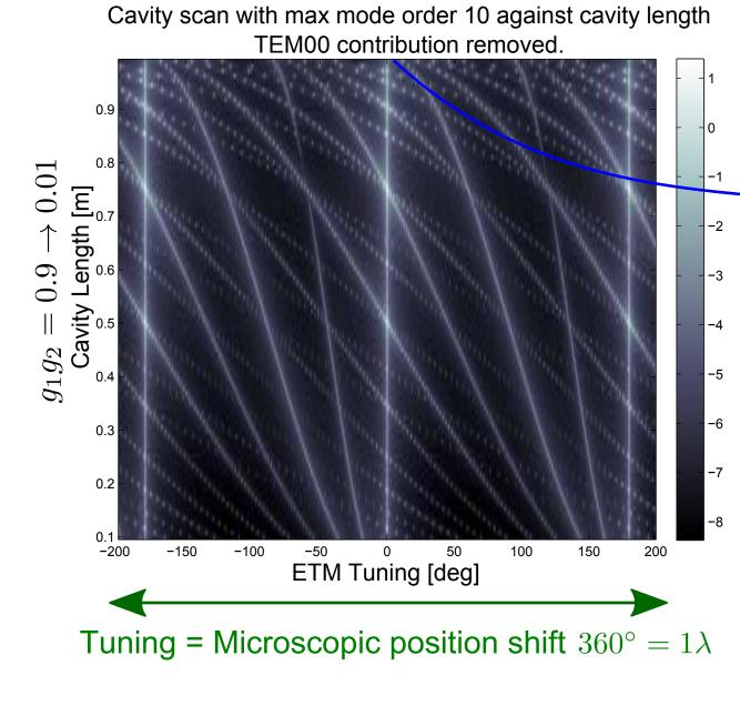
As  $g_1g_2$  tends to instability i.e. 1 or 0, the HOMs bunch together as the separation frequency is on the order of the Free Spectral Range (FSR). This mode bunching ruins error signals as seen on th left and can make the cavity inoperable even before it has reached instablity.
