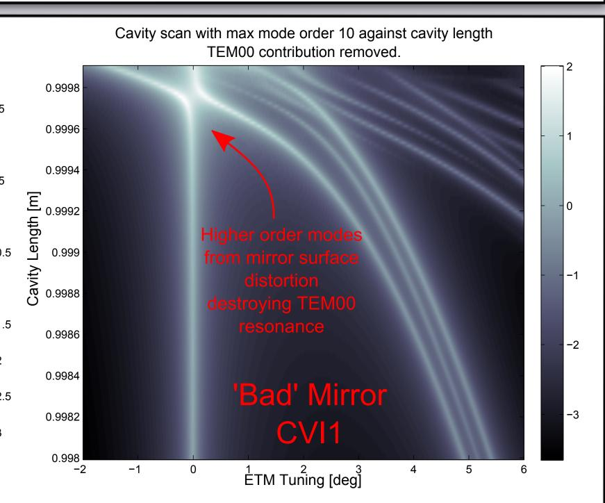
It was found that the difference between many of the good and bad mirrors was minimal and likely the differences would not visible in our experiment. One mirror, CVI1, appeared the worst and resulted in greater round trip losses which will likely provide a visible difference.
