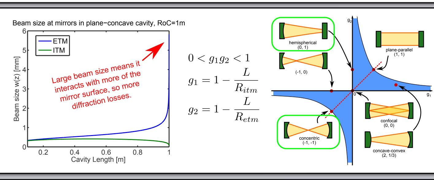
Beams resonant in cavities near Near-Instability have large spot sizes. This has the advantage of reducing the effect of mirror coating brownian noise by averging over a larger surface area.
