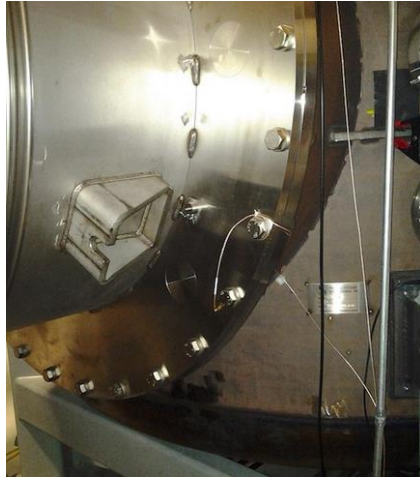
Figure 1: An Accelerometer fully mounted on a chamber
