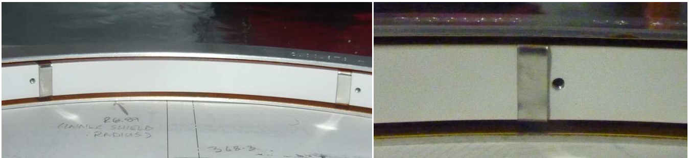
Figure 10. Hand-made metal clips used to locally reduce the emissivity of the UF RH. They turned out to be a convenient way of correcting the heating profile and reduce the residual astigmatism.
