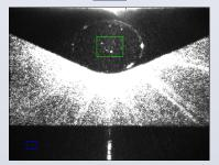
♦ This figure displays the Output Mode-Cleaner optic with noticeable scatter. The green box surrounding the scattered light on the surface is our Region of Interest (RoI).
