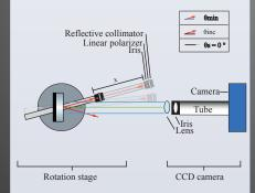
♦ The figure above shows both our scatterometer prior to change and, shown with a fading finish, the scatterometer with the amendment of moving back the iris, polarizer, and collimator back ~25cm to achieve an incident beam angle of 4 degrees. A technique called "Drag Wiping" was used to reduce the scatter on the Output Mode-Cleaner. Drag wiping consists of lightly damping a cloth with methanol, which then is carefully applied onto the optic so that it sticks, and then dragged off the mirror
