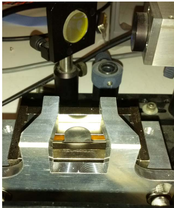
Figure 4 beam blocking tab is visible between the aluminum forks in the foreground
