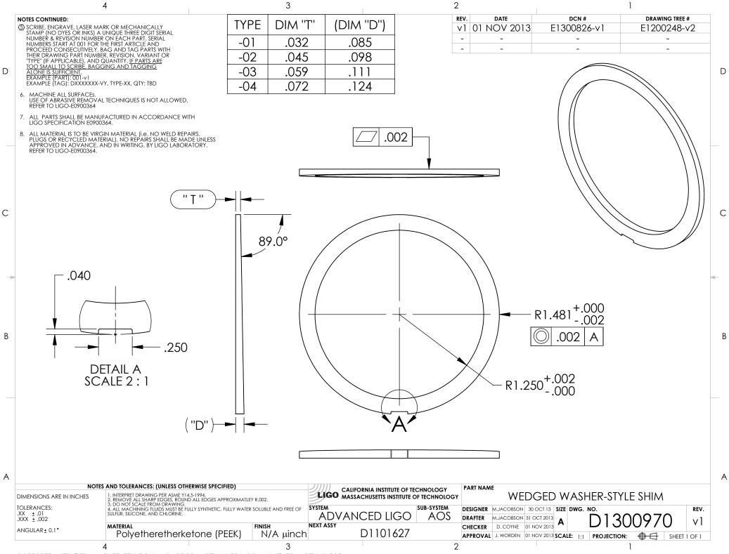
D1300970\_WEDGED WASHER-STYLE SHIM, PART PDM REV: X-004, DRAWING PDM REV: X-002
