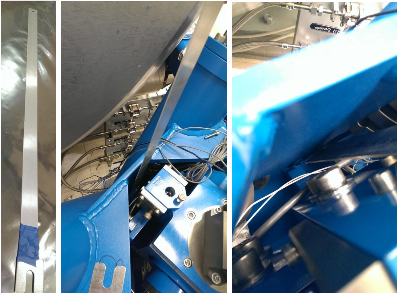
Figure 12: First gap to measure (on the first picture, we can see the tool used to measure that gap)
