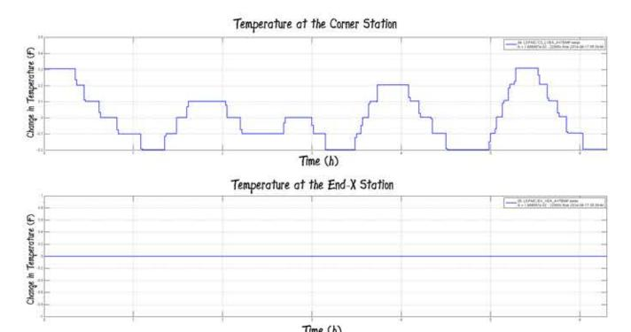
Temperature fluctuates with roughly 30 min period, yet transmitted power takes 2-4 hours to decay.
