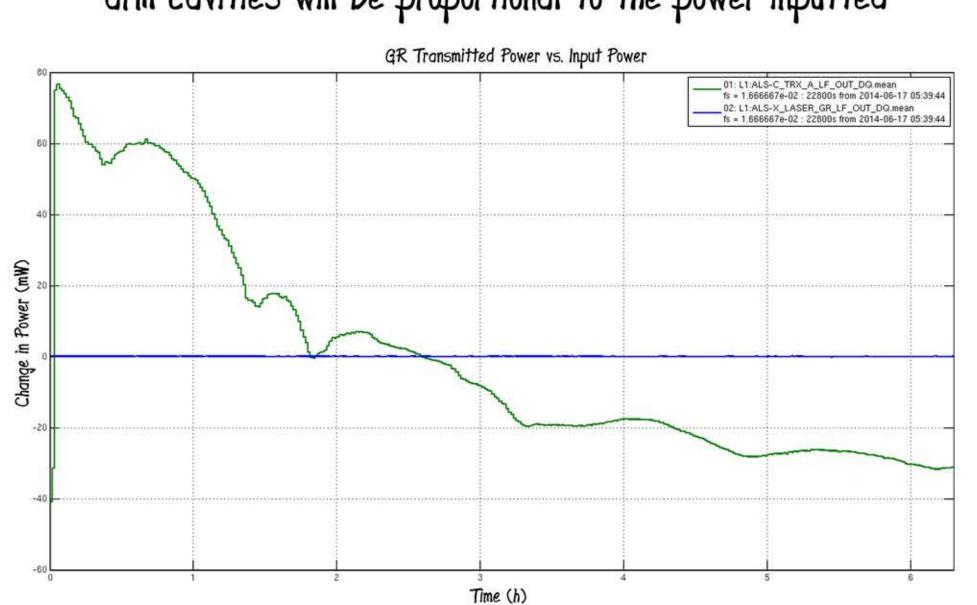
This plot shows the power from the laser vs time on Tune 17th. It can be seen that the power does not decay, so we can rule out the input power.
