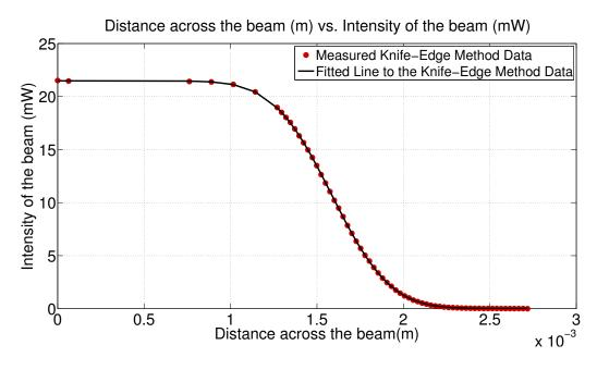
Figure 3: One set of measurements taken using the knife-edge method after they were fitted to the Gaussian error function.
