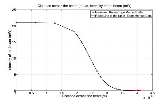
Figure 4: One set of measurements taken using the knife-edge method after they were fitted to the Gaussian error function.
