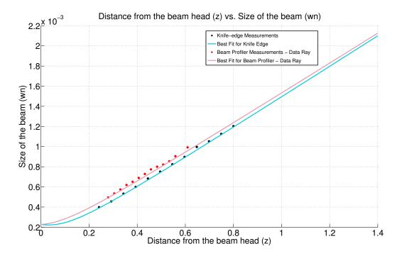
Figure 5: Graphical results showing a comparison of the constructed beam profiles from the measurements taken through the knife-edge technique and through using the beam profiler.
