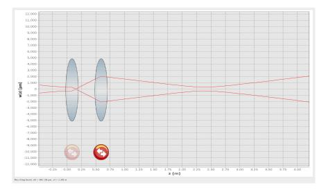
Figure 6: One of the designs for the mode matching telescope using the "Jammt" software.
