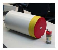
the tube. Tape the balloon to the tube (that's yellow duct tape you see in the photo).
