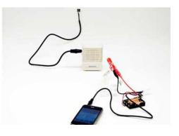
• You'll use the MP3 player to play some music. The MP3 signal will go onto the laser light, onto a light sensor and into the speakers. Students can interrupt the laser beam and turn off the music.
