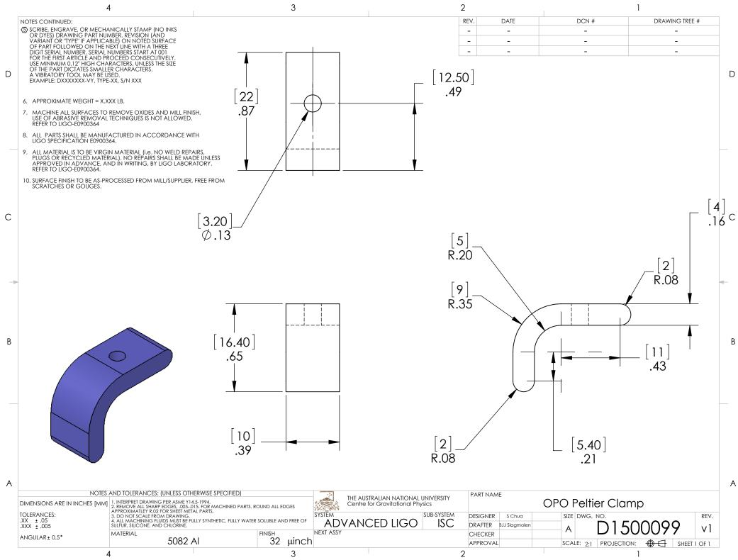
Peltier Clamp, PART PDM REV: , DRAWING PDM REV:
