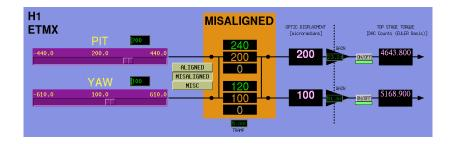
A single channel/slider can be used to control the current offset value, with a switch to select which alignment state the current value corresponds to.
