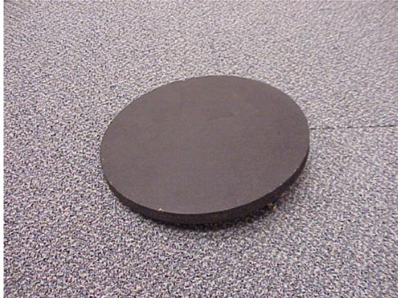
You will need a flat piece of particleboard (or other material) on which to mount the parts. A 1-ft diameter particleboard "round" was used purchased from a local hardware store for this demo. The base plate needs to be smooth and flat to make mounting and adjusting parts easy. We painted our base plate with a thin coat of flat black paint for purely cosmetic reasons. (Do not spoil the flatness with a thick, crummy paint job!)
