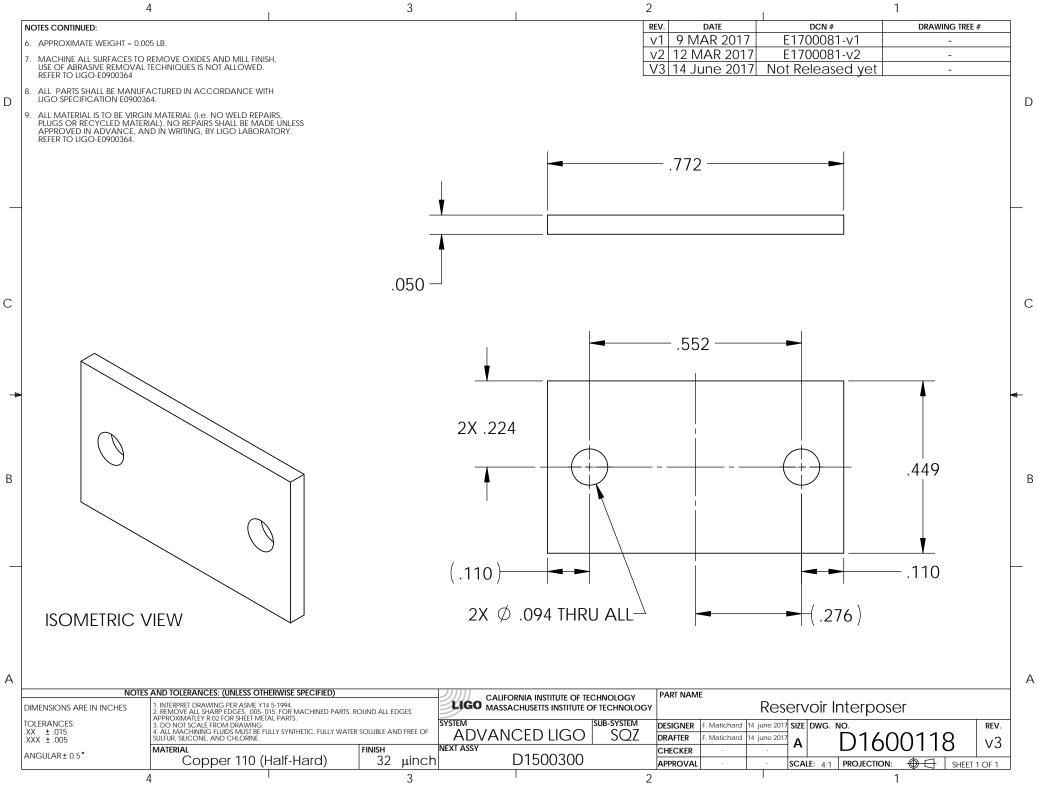
D1600118 aLIGO VOPO Reservoir Interposer, PART PDM REV: X-009, DRAWING PDM REV: X-003
