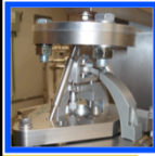
Inductive aLIGO Pre-isolator Stage
