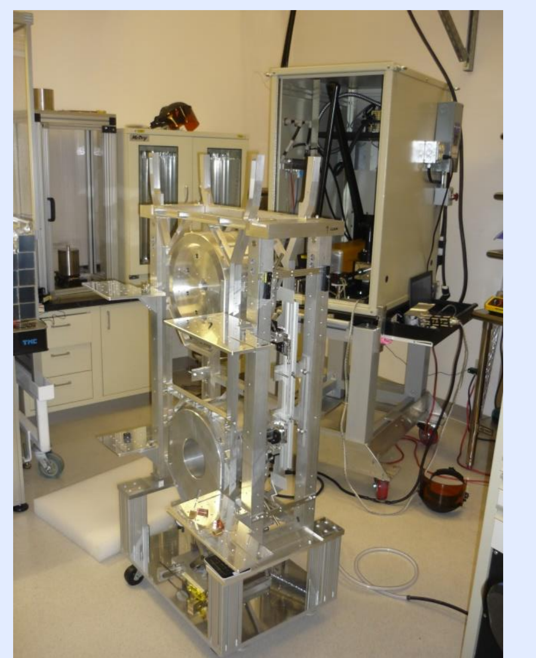
Figure 7: Suspension with thinner fibres installed at LHO (April 2015)
