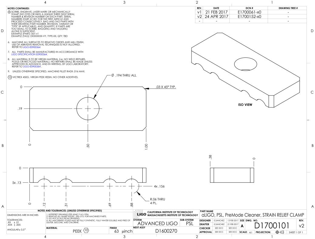
D1700101 aLIGO, PSL, PreMode Cleaner, STRAIN RELIEF CLAMP, PART PDM REV: X-002, DRAWING PDM REV: X-006
