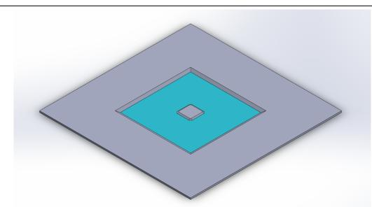
The etching process leaves an exposed 100 nm thick membrane with an island of Silicon in the center. The size and shape of this island mass can be altered with the masking design. SiN
