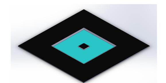
A masking (black) is applied to prevent frame and mass from being etched away
