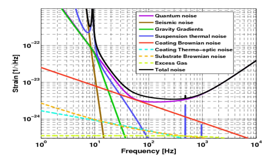
Coating Brownian noise is a fundamental noise in the detection of gravitational waves (GW).
