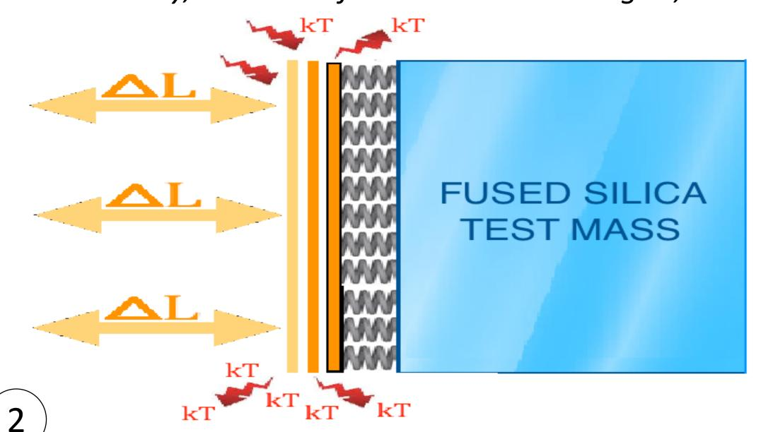
Optical coatings on the GW detectors test masses behave as though they were attached to the substrate by springs. When random thermal energy exchanges distort them there will be an effective length change in the laser cavity.
