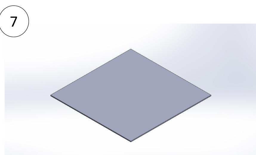
We take advantage of the manufacturing process to leave a mass of silicon in the center of the membrane. A 100 nm layer of Silicon Nitride is deposited onto the bottom face of a wafer of silicon (grey).
