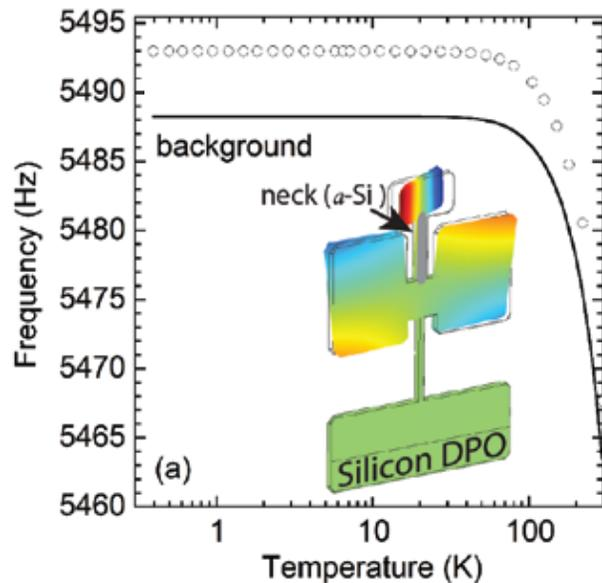
Measure resonant frequency and internal friction (damping)  $Q^{-1}$  of a double paddle oscillator (DPO) as a function of  $T$  before and after depositing a film
