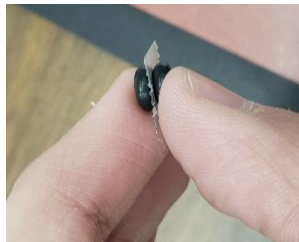
Figure 5. Viton stack, attached using double-sided tape.
