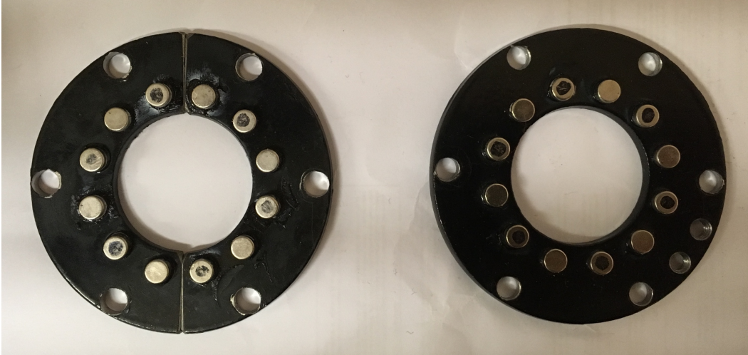
Figure 10. Image of the left and right disks. Black dots were applied with markers to indicate the North Pole of the magnet. One disk is cut in half for assembly reasons. The soft iron acts as a magnetic flux return confining the magnetic field to that which occurs between facing magnets.
