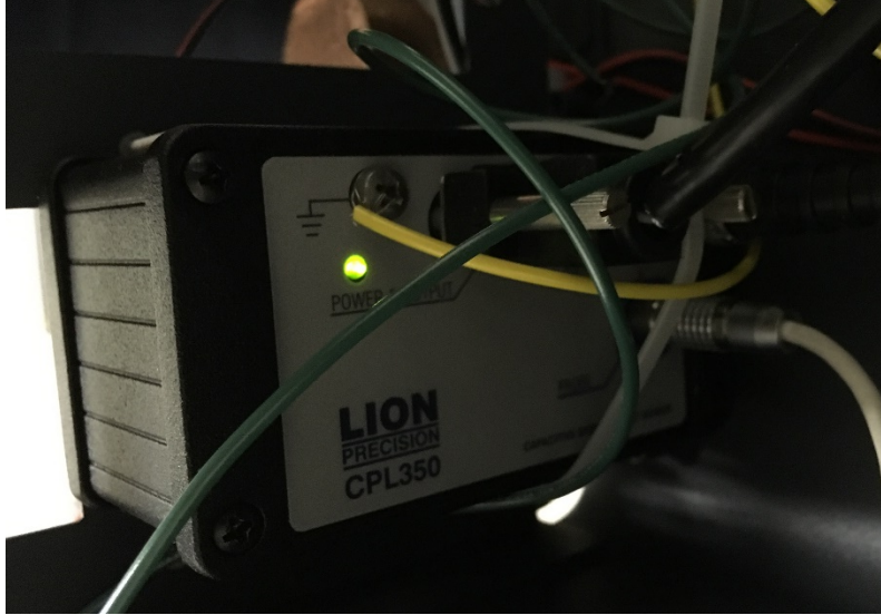
Figure 81. Electronics used to control the capacitive sensor.
