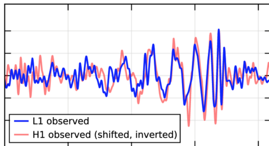
FIG. 2. Strain ( h(t) ) plotted against time ( t ) for GW150914, LIGO's first GW detection. L1 is the data from the Livingston, Louisiana detector; H1 is the data from the Hanford, Washington detector. Figure from [6]
