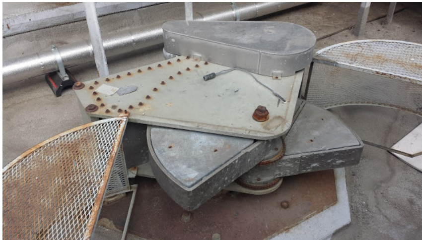
Figure 7: The sinusoidal shaker at the top of Milikan Library
