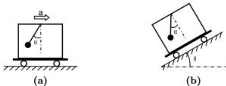
Figure 1. Simple pendulum in a box as a horizontal inertial sensor. The sensor is sensitive to both horizontal acceleration (a) and tilt motion (b), which demonstrates the intrinsic tilt-horizontal coupling problem for inertial horizontal sensors.
