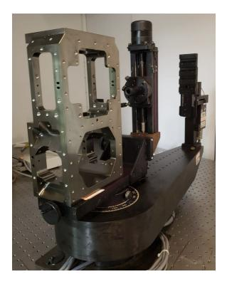
Figure 3. HDS structure on Scatterometer. The first set of measurements were taken with this configuration. For future measurements, the laser was pointed at another surface on the structure.
