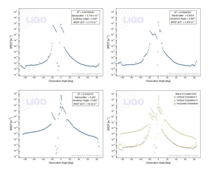
The vertical orientation plots both have very strange dips near the top of their curve. This is likely due to some calibration error on the scatterometer. The HDS structure will be measured again in the vertical orientation to obtain better data
