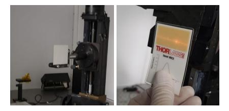
Figure 2. Aluminum sample in scatterometer (left) and laser beam profile after hitting the sample (right). The uncoated sample and HDS structure distort the laser beam in a similar way.
