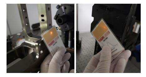
Figure 1. Laser beam profile before (left) and after (right) hitting the black Ni coated HDS structure. The beam profile changes from a clearly defined point to a horizontal line.
