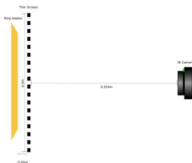
Figure 2: Optical Diagram of the In-Air IR Test Facility Setup
