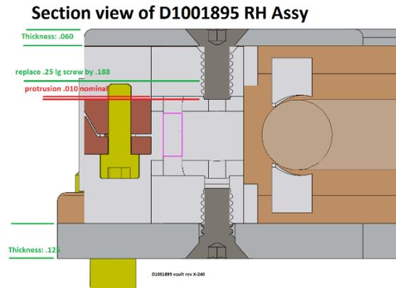
Figure 10: Image from FRS Ticket 4552 [9] that shows the inside of the ceramic macor retainer. The dark grey structures on the top and the bottom of the image are the screws in question.
