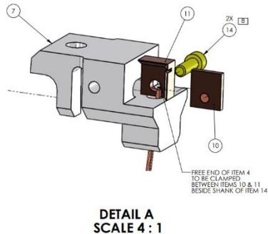
Figure 4: Image of one of the end pieces. The white structure is the ceramic macor retainer and the brown structures are the copper clamps [4].
