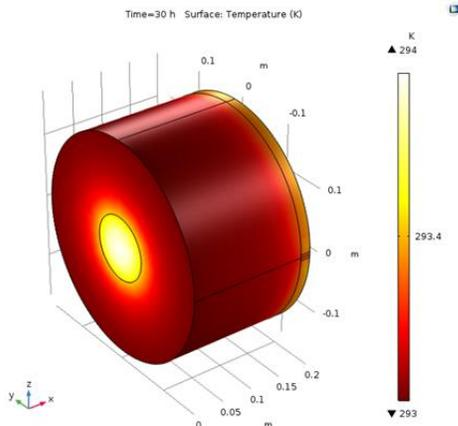
Figure 14: Temperature model of the test mass with the current ring heater design. On the front is the laser and on the back is the ring heater.
