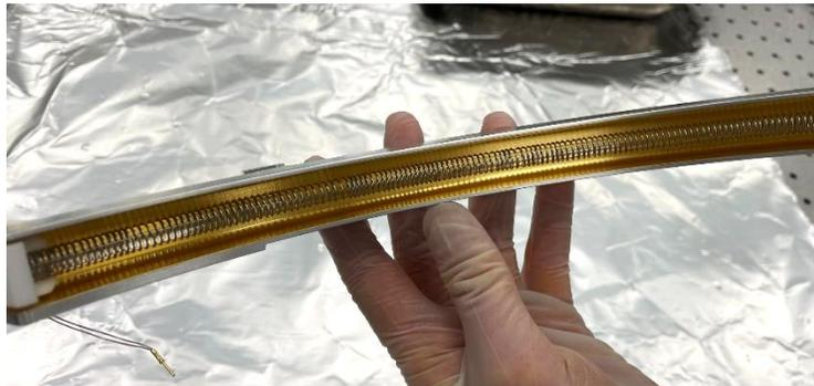
Figure 3: Image of the inside of one half of the ring heater. The heating element and gold painted interior of the shield are visible.
