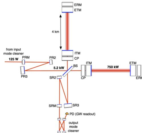
Figure 1: A simplified diagram of the interferometer. The Y arm goes in the y direction (vertically), while the X arm goes in the x direction (horizontally) [2].
