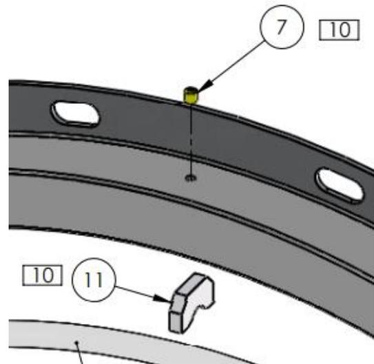
Figure 7: Image of the midspring's predecessor, the midspan. Item 11 is the midspan itself and item 7 is the metal set screw [6].
