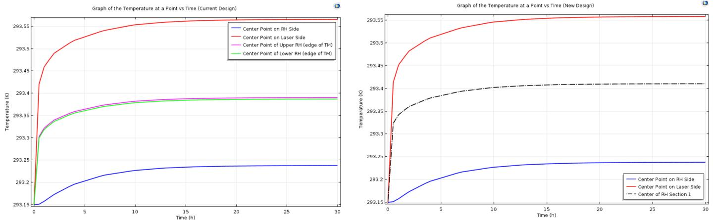
Figure 17: Graph of the temperature of the current (left) and new (right) ring heater designs. There is very little variation between the two.
