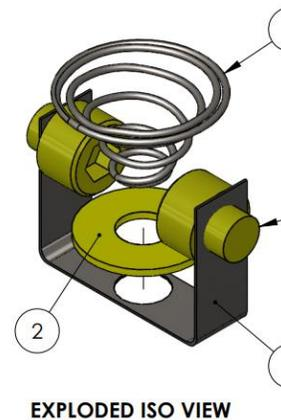
Figure 5: Image of the midspring. The yellow structures are made of ceramic, while the grey is made of metal [5].
