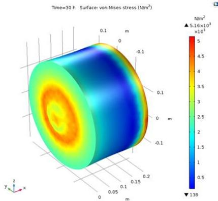
Figure 12: Stress model of the test mass with the current ring heater design. On the front is the laser and on the back is the ring heater.
