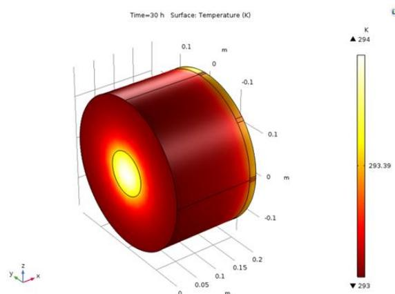
Figure 15: Temperature model of the test mass with the new ring heater design. On the front is the laser and on the back is the ring heater.
