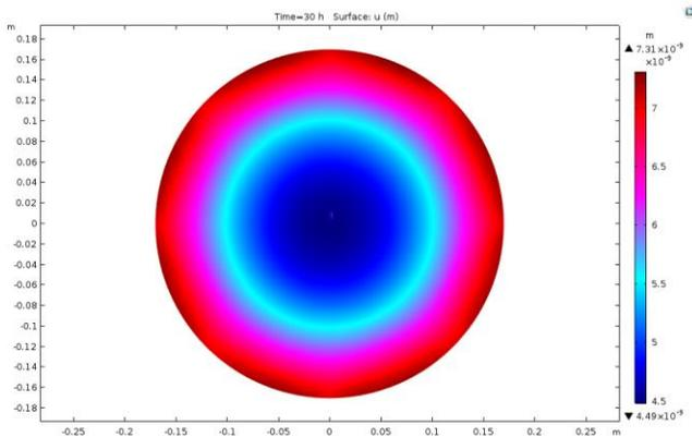
Figure 19: Image of the displacement of the test mass from the original model of the new design caused by heat deformation. Red indicates more displacement and blue indicates less displacement.
