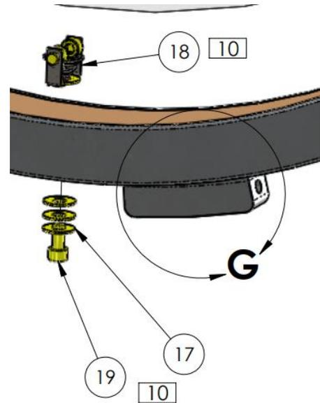
Figure 6: Image of the midspring (left) and the temperature sensor (right, labeled "G"). Item 18 is the midspring structure, while items 19 and 17 are the ceramic screw and washers respectively [4].
