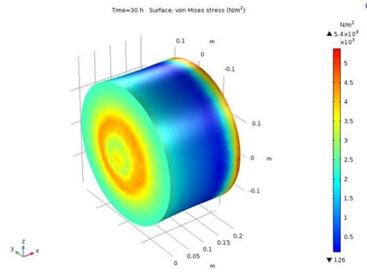
Figure 13: Stress model of the test mass with the new ring heater design. On the front is the laser and on the back is the ring heater.
