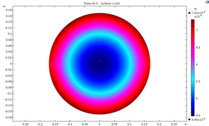
Figure 18: Image of the displacement of the test mass from the original model of the current design caused by heat deformation. Red indicates more displacement and blue indicates less displacement.
