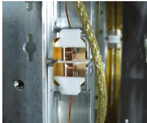
*Figure 9: Image from LHO alog 12229 [8] that shows how close the copper pieces are when the RH is installed, and they've been built correctly*
