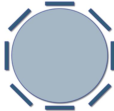
Figure 11: A basic drawing of the suggested 8-sided design. The large circle in the middle is the test mass, and the darker rectangles around it are the ring heater sections.
