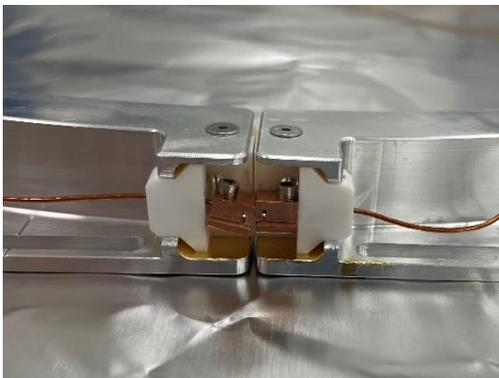
*Figure 8: Example of how the copper clamps can touch.*
