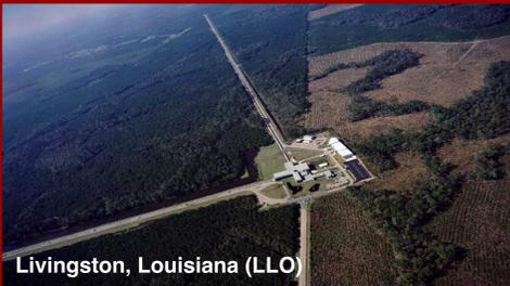
To make this detection, incredible precision is required. LIGO's interferometers are the largest ever built as the size is crucial to detecting gravitational waves. The longer the arms of an interferometer, the smaller the measurements able to be made. Its 4 km arms allow LIGO to detect a change in distance 10,000x smaller than a proton.
