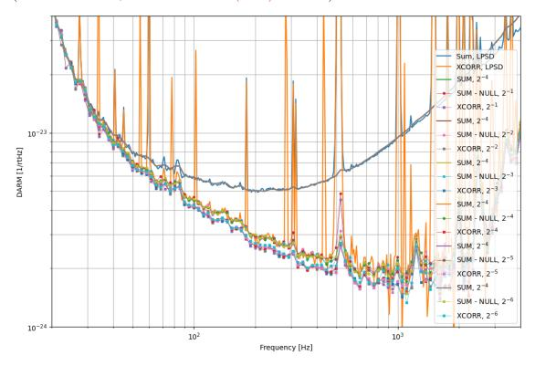
As shown in the plot above, the rebinned SUM - NULL traces are consistent with LPSD results, but the rebinned scipy.signal.csd traces don't follow. This problem doesn't improve when we increase the spectral resolution. It's a systematic error introduced during the rebinning of the xcorr spectra. The difference between the SUM and Sum, LPSD at high frequencies are due to the known cailbration problem in PD time series. It doesn't affect the discrepancy at low frequency.
