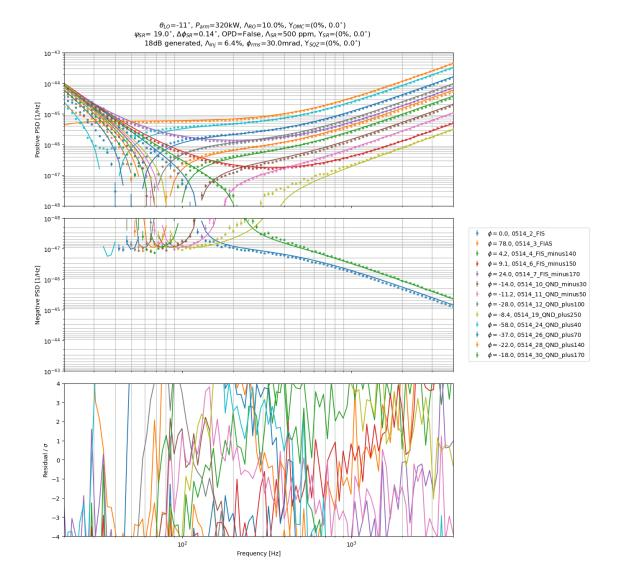
This plot shows a model without MM that fits the DARM difference at high frequencies. It fits positive (non-QND) squeezing angles quite well. However, it is quite far away from the low-frequency part of the negative (QND) squeezing angles while fitting the high frequency part. This is especially problematic for -58 deg case where the low frequency dip at around 35 Hz was totally missing. Mode-mismatch can perhaps accomplish the broadband fitting.
