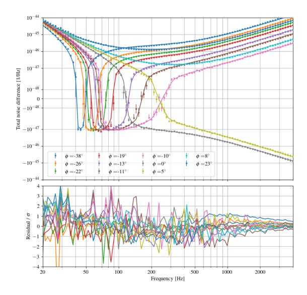
This is our best model that is able to minimize residuals for all FIS. The inferred results are also summarized in the table above. Notably, the arm power is inferred to be around 260 kW instead of 300 kW calculated from PRG. Since we don't have other data that directly measures arm power yet, we will use 260 kW.
