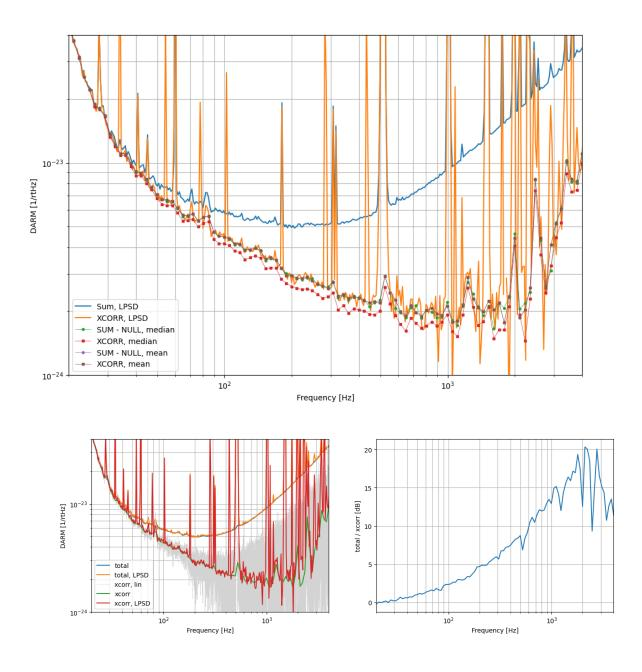
Both scipy.signal.csd and LPSD are consistent. The classical noise at 1 kHz are around 15 dB (5.6) lower than total noise.
