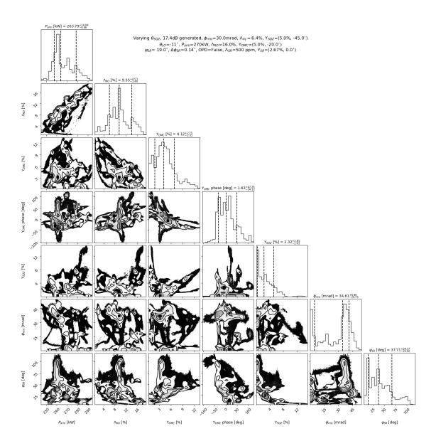
The final likelihood is 10144, slightly higher than Gaussian-distributed walkers. We should use a flat-distributed walkers for more explorations.
