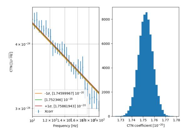
This is the MCMC where we infer the magnitude of CTN coefficient. The distribution of the result is pretty Gaussian which is good. However, the slope doesn't look correct. We can also fit it with slope as another free parameter.
