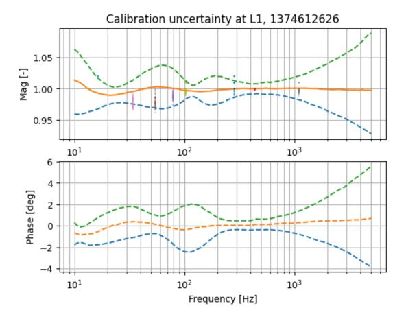
The monitor lines are lower than medians by 2% at 33.93, 54.17, and 78.23 Hz. When we multiply the median curve with the correction, the new envelope is correct and contains the uncertainty of monitors (see Ling Sun's comment).
