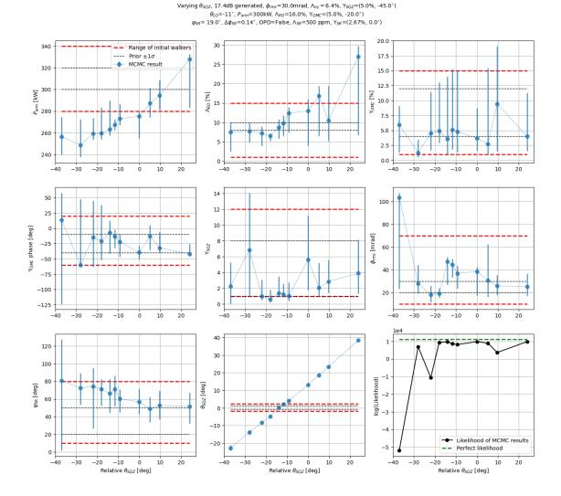
It's very interesting that we have an outlier of arm power at squeezing angle of 24 deg. Although the inferred arm power is much larger than other cases, the MCMC results give a better posterior than initial settings. It could be a case where the random starting points of all walkers are very bad so none of them converge. But I run a second MCMC and it gives the same result. Both of them yield much lower posterior than inputs.
