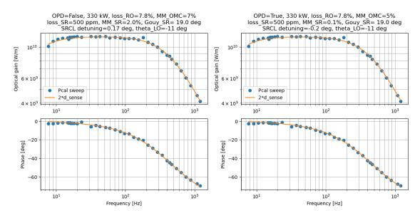
There's a factor of 2 difference between the gwinc model and measured optical gain. We've compared the optical gain with another simulation tool o\_O and they match relatively well. We will still fit the offset difference anyway.
