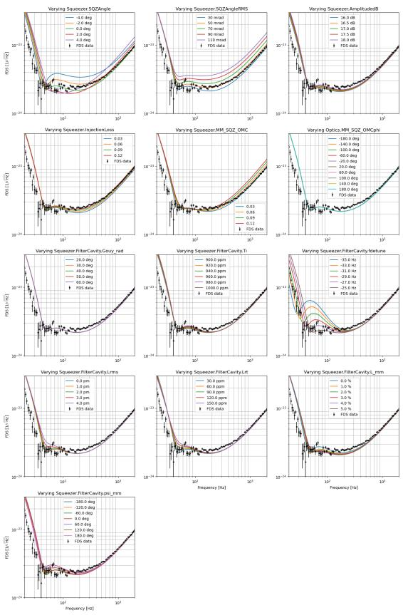
These parameters above are only affecting the squeezing system, and not IFO. We only want to change these to not affect the inferred FDS data.
