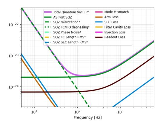
The shot noise is the sum of "AS Port SQZ", "Readout Loss", and "Mode Mismatch". The QRPN is "SQZ misrotation". In fact, the quantum noise can be understood as a single quantum mode that experiences frequency-dependent ponderomotive squeezing from interferometer, which is how gwinc models it.
