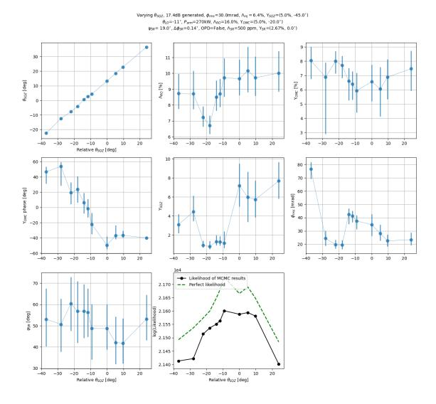
The readout loss has less dependencies with squeezing angle after we fix the arm power. The IFO parameters like  $\Upsilon_{OMC}$  and  $\psi_{SR}$  vary a little bit to the squeezing angle, which is promising to us after we set them to be common parameters.
