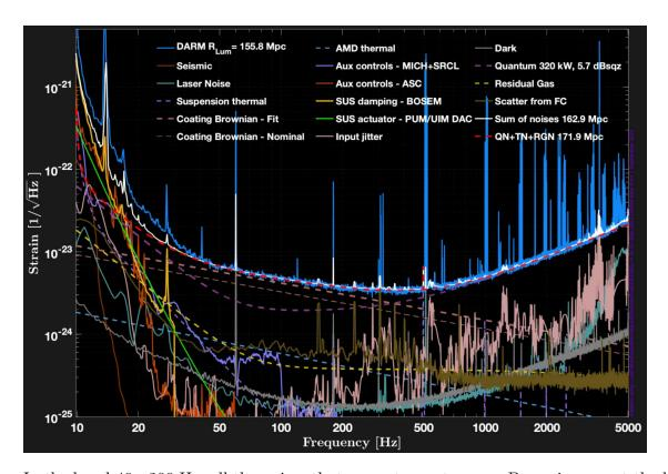
In the band 40 - 200 Hz, all the noises that are not quantum nor Brownian are at the level of 1e-24. They are 3 times less than Brownian noise, so our over-estimation of Brownian noise is maximum 10% at 200 Hz and less at lower frequencies. Knowing the shot noise, we can have a band of possible QRPN:
