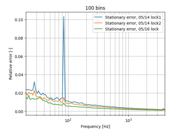
The stationary error in lock2 is lower because it has 50% more unsqueezed DARMs than lock1. Same story with 05/16 lock. Note the scatter noise at 80 Hz is less in the second case. It is because the scatter noise is stationary, not because we had lower scatter noise.
