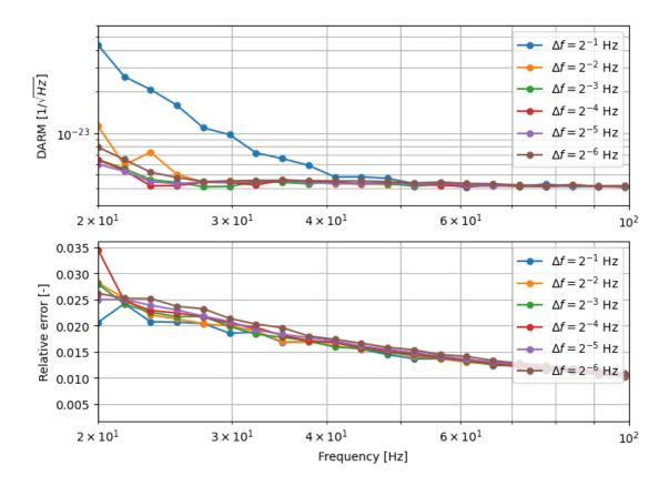
The relative error is set to the PSD error before rebinning. The rebinned relative error doesn't depend on the spectral resolution, which makes sense. As we increase the spectral resolution, we have less averaging so the statistics are not enough. There's a trade-off in the resolution selection, and we pick  $2^{-4}$  Hz to balance the trade-off.
