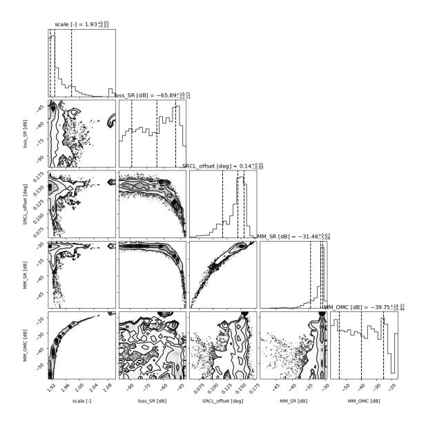
In the case where thermal lensing is negligible, the MCMC constrains the scale and SRCL detuning pretty well. Other parameters like losses and mismatches are not well constrained
