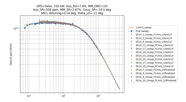
Both sensing functions measured in two different ways agree pretty well, along with the model curves. The DC level is still questionable, as the scale factor 1.93 can't be easily absorbed into the arm power of 330 kW.
