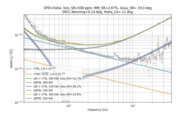
As we can see here, the QRPN is below 5% of coating Brownian noise PSD between 60 - 200 Hz, even with the highest arm power possible of 360 kW. Besides QRPN and shot noise, there is also other classical noise there, for example, scatter noise at 80 Hz and FC backscatter noise with the magnitude of 7e-25. Therefore, we can safely infer CTN with the frequency band of 100 - 200 Hz. The other classical noise there will not lead to more than 5% overestimation of the coefficient.
