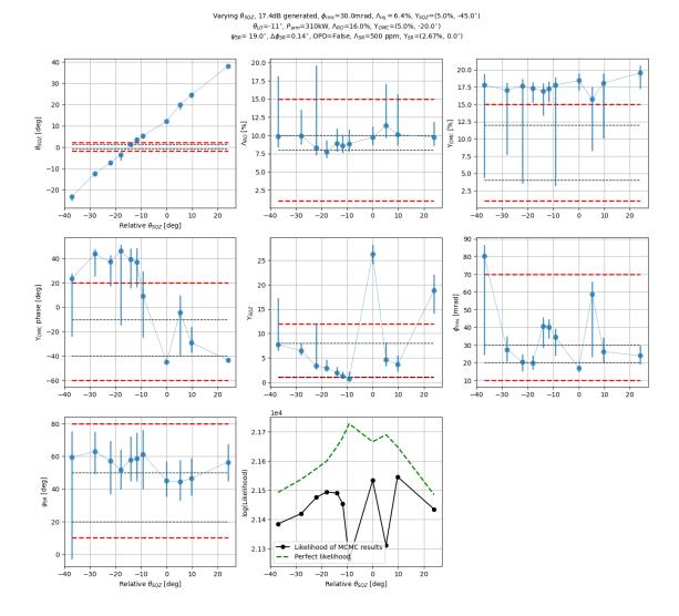
Leave calibration error out of rebinning and using more bins (100) increases the errorbar. In this case, the default parameter is already pretty good, and MCMC doesn't improve everything by too much. The calibration error is largest at high frequency, whereas we need it to be larger at low frequencies.
