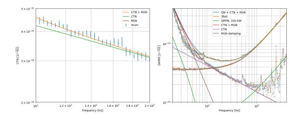
The residual gas damping noise can be elevated to fit the measured DARM at 100-200 Hz, but it doesn't make sense at low frequencies. We can't fudge the excessive residual gas noise to explain the steeper slope of the xcorr noise there.
