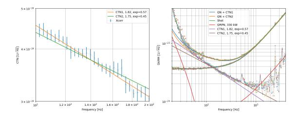
The MCMC curve with slope as a free parameter gives a better fit to the data. However, it predicts an exponential of 0.57, which is more than  $0.45 \pm 0.02$  used in PRD 103, 072001.
