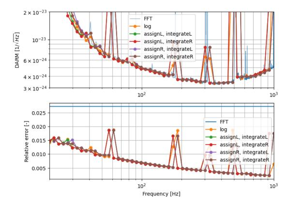
Comparison of various FFT resolution and the rebinned results. The  $\Delta f = 2^{-4}$  Hz is minimally required to correctly estimate PSD at low frequency. However, the spectral resolution affects the accuracy of low-frequency PSD and especially the subtracted noises.
