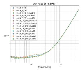
The shot noise of FIAS and near anti-squeezing have weird bump around 150 Hz. This is perhaps because the increasing of quantum noise that reduces SNR of calibration lines. Luckily, the anti-squeezing spectra are not very sensitive to many parameters, which will be shown later.
