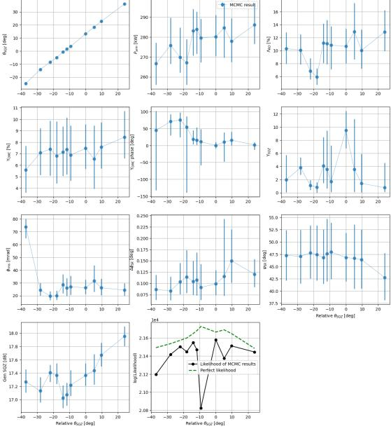
The inferred squeezing angle is shown to be linearly correlated with input squeezing angle, which makes sense because it is the parameter that we actively change to get various FIS data. There is a DC difference between two angles, namely  $\theta_{SQZ} = 0$  (phase squeezing) corresponds to ~12 degree in gwinc model. This is due to the non-zero LO angle and other phasing degradations.
