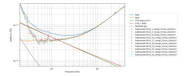
The subtracted DARM contains quantum noise plus classical noises that are not CTN. The difference between two CTN models are less than 8%. We will use the CTN model with AMD correction.
