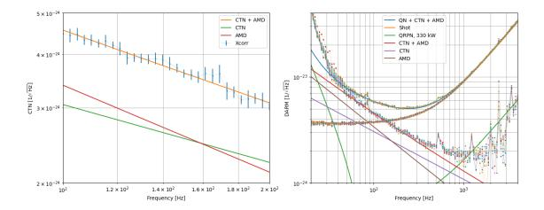
The difference between measured DARM and total noise budget is also smaller with the addition of AMD.
