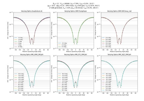
The free phasing parameters doesn't change the shape nor the magnitude of the DARM difference. The  $\Upsilon_{OMC}$  phase will change the magnitude by more than 10% near anti-squeezing, but it doesn't change much between -40 to 40 degree.
