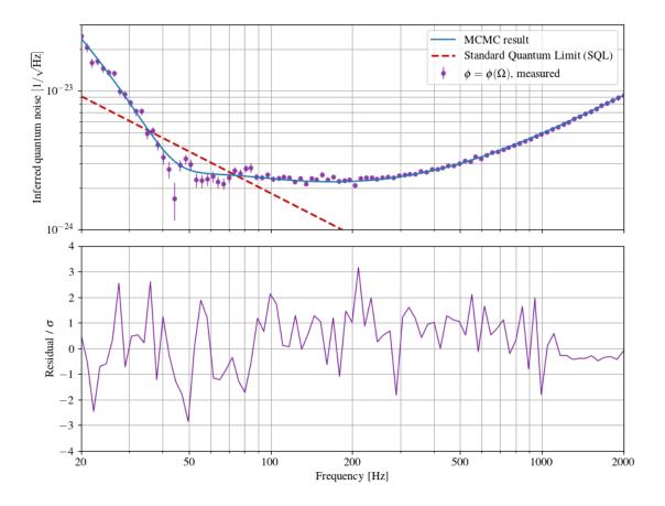
The total uncertainty of the FDS data is shown below. The error sources have been explained in the previous sections. The FDS quantum noise is seen below standard quantum limit by up to 3 dB at 50 Hz, while maintaining squeezing at high-frequencies. This marks LIGO as a quantum nondemolition gravitational-wave detector (KLMTV).
