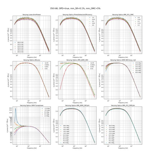
These plots show how the sensing function from gwinc is affected by ifo parameters. The title shows the canonical parameter set where we perturb from. For each subplot, the title says the perturbed parameter. The various values of such parameters are labeled in the legend. The sensing function is therefore very sensitive to  $\Upsilon_{SR}$ .
