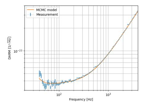
The MCMC on unsqz quantum noise only constrains the SRC Gouy phase. All other parameters are not well localized. This is because both the measurement doesn't have the sharp feature that MCMC can extract and the uncertainties are large. The model is plotted here with the data.
