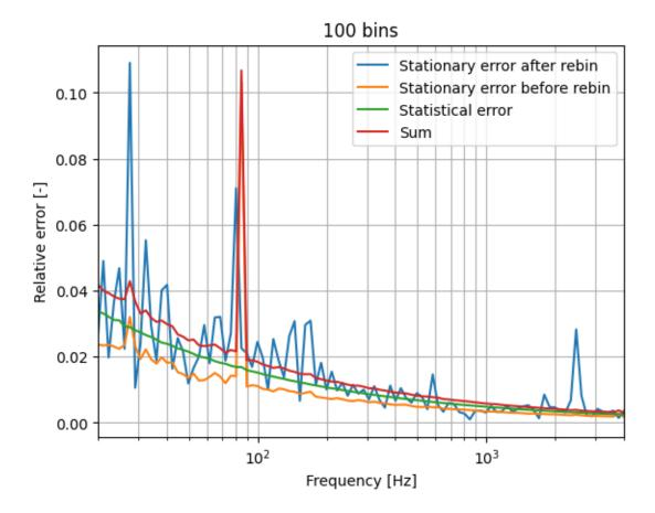
If we rebin DARM first, the statistical uncertainty would be suppressed at high frequencies while the stationary error shouldn't change, assuming the stationary error has enough bandwidth to not be averaged out by rebinning. This is the blue trace, which still resembles the statistical error. We only know that the 80 Hz peak is scatter noise and non-stationary, the rest is hard to tell if its stationary or not.
