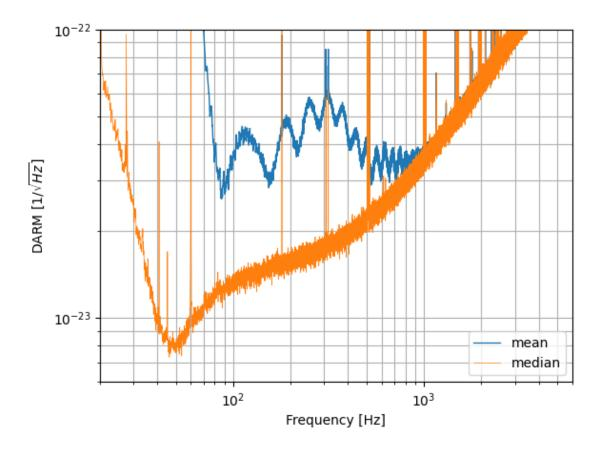
As seen in the plot, the mean statistics is heavily affected by the glitch whereas median is less affected and captures the sub-SQL dip at 50 Hz.
