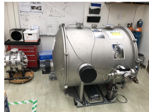
Caltech Vacuum Chamber with Hartmann Wavefront Sensor ( G2400546 )
