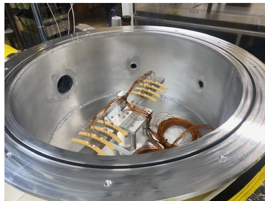
Heater Elements in UCR Vacuum Chamber ( G2400546 )
