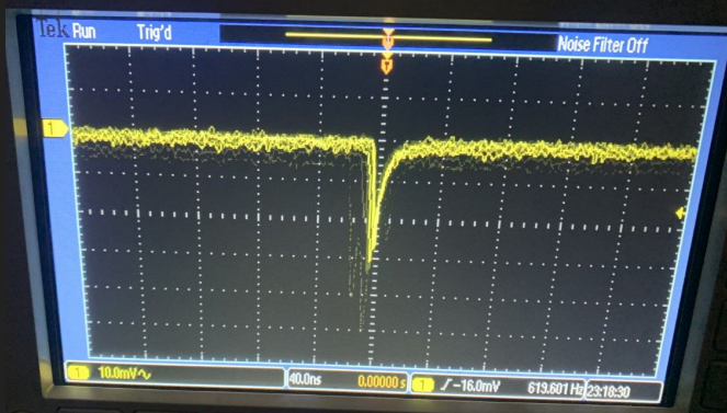
PMT in oscilloscope on nanosecond timescale
