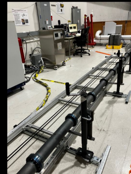
Progressive induction heating bakeout
