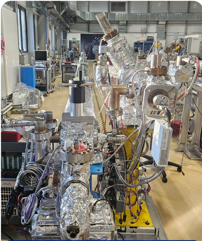
LoLA (Low outgassing Large Apparatus) Full DN250 - 16 m vacuum system.
