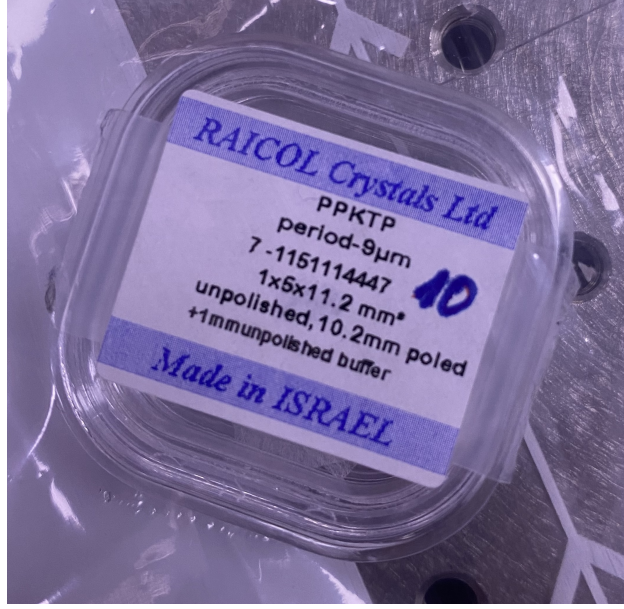
Figure 4: A container of ANU preloved crystal. Note crystal was subsequently polished by Photon Laseroptik, with a wedge added to one end and then AR coated by Laseroptik.
